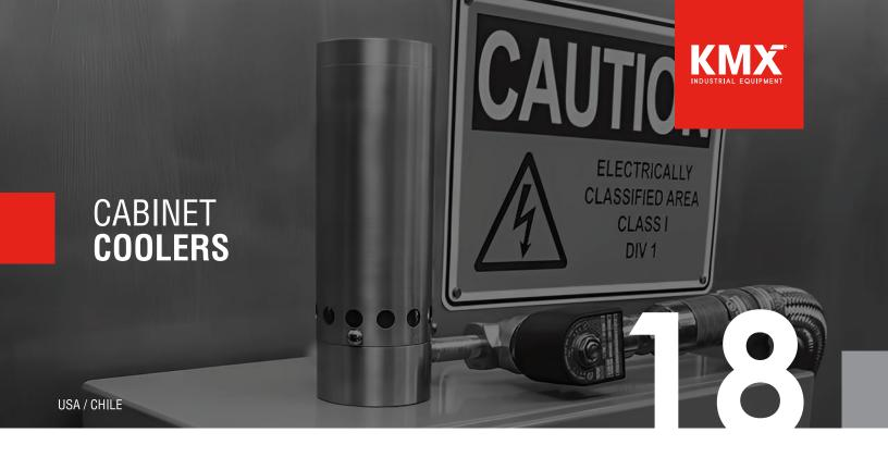
Industrial cooling and cleaning system for electrical cabinets and panels equipped with Vortex tubes from the Canadian brand Nexflow. These tubes allow the injection of an extremely cold air flow into the cabinet, reducing the temperature and creating positive pressure inside, preventing the entry of dust and the risk of a short circuit.
